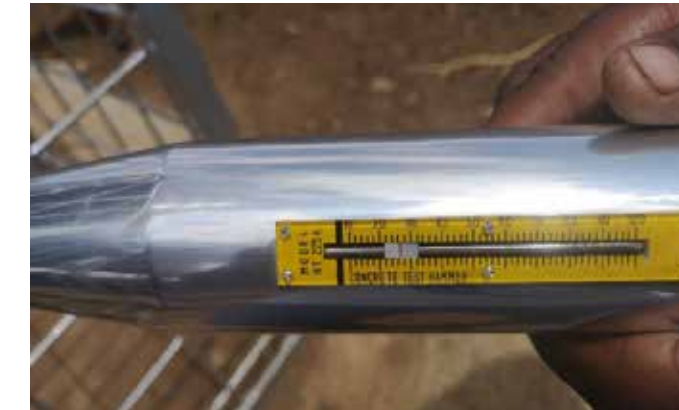
Concrete strength test showing 27mpa, well above the required 20mpa
