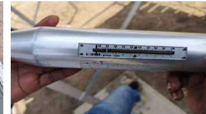
Concrete rebound hammer tester
